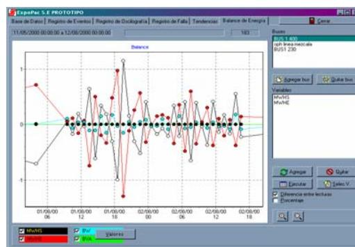
This graphic environment helps visualize losses in the substation and efficiency of the transformation process under the different circumstances analyzed.
