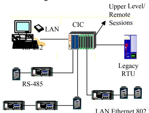
The CIC is based on Motorola Computer Group's embedded boards on a PC/104 platform: a pentium single board computer @ 350 MHz, 64 MB RAM. It has RS232/485 serial port for configuration, a parallel port to support a printer, keyboard jack and optional 3" floppy drive.
