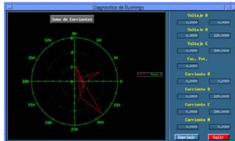
The above example is a bushing sum of currents polar graphic. Graphs are also configurable to the user's liking.
