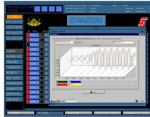
Downloads can be done by setting a trigger if a certain variable reaches "x" value and/or by programming it on a timely basis and/or by operator request.
